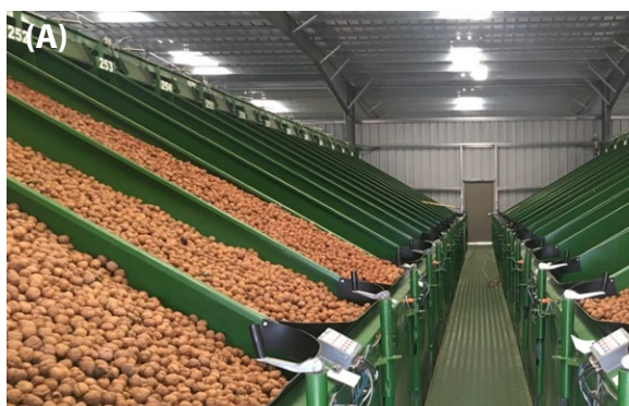
FIG. 1. (A) A California walnut drying facility with stationary bin dehydrators. (B) Stationary bin dehydrator schematic; arrows show the flow of air.
