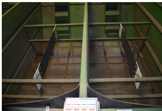
Two empty walnut drying bins with in-bin moisture meters (IMM) installed at the center of each bin. The perforated bin floor is visible, supporting uniform vertical airflow through the walnuts during drying. Photo: I.R. Donis-González.
