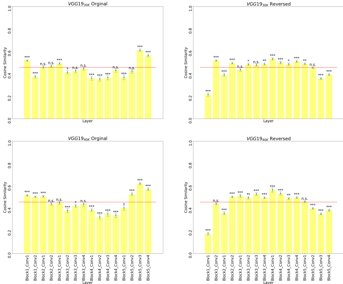
Figure 5: Cosine similarities between the saliency maps (or their reverse) at different convolutional layers and the human participants’ attention heatmaps. Error bars represent standard errors. The red horizontal lines represent the baseline cosine similarity (i.e., mean cosine similarities between human participants’ attention heatmaps and randomly generated heatmaps). On each layer, we ran a paired t-test between the observed cosine similarities and the baseline cosine similarities (* < .05; ** < .01; *** < .001).
