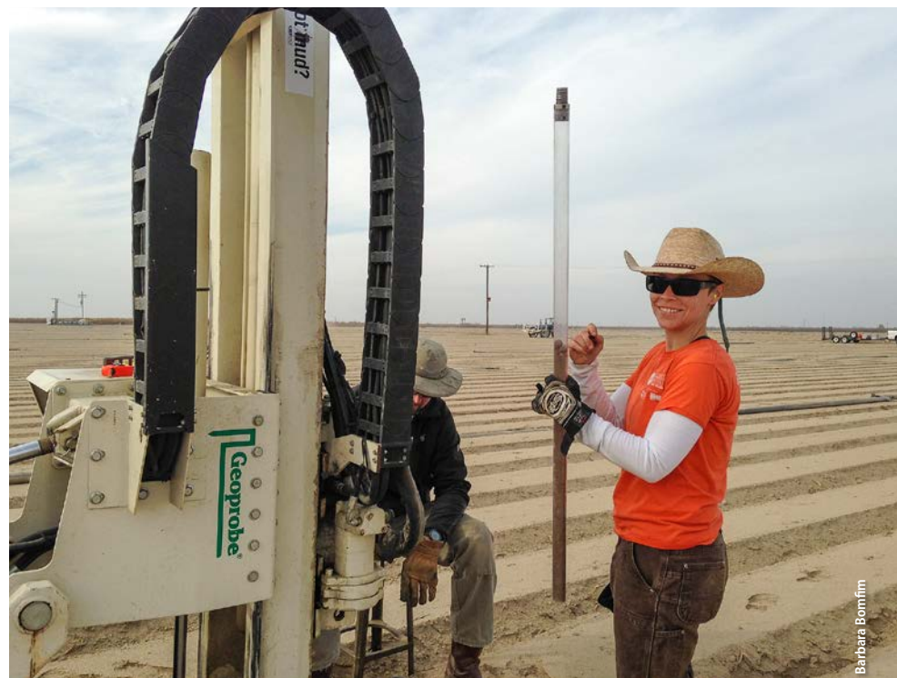
A Geoprobe push-drill system was used to collect soil cores to 30 feet in depth in fields planted in almonds, tomatoes and wine grapes in the Kings groundwater subbasin.
