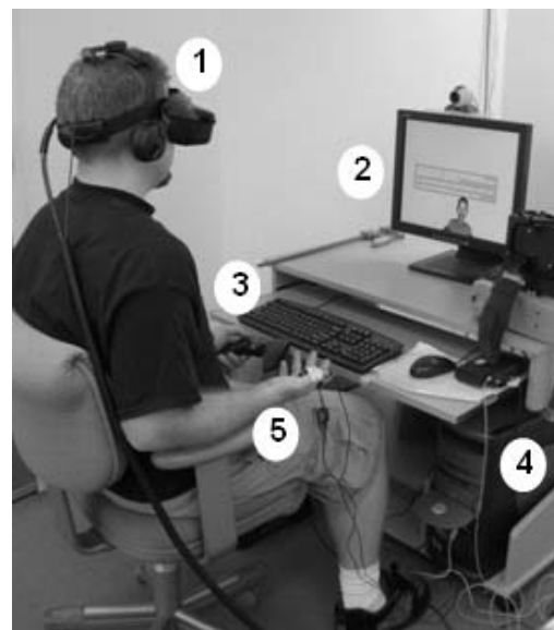
Figure 2: Participant in VR learning environment: 1) Head-mounted display (HMD) and orientation tracker, 2) monitor showing the experimenter what the participant sees in the HMD, 3) Game pad used to notify agent/avatar, 4) rendering computer, 5) equipment recording skin conductance level.
